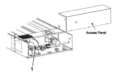
2. Remove the #6 screws and nuts holding existing module. **Note**: The screws and nuts will be re-used to attach the new module. Remove module from control cabinet.
